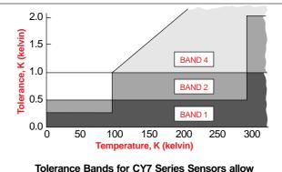
Tolerance Bands for CY7 Series Sensors allow selection of appropriate (and economical) accuracy levels for a given application.
