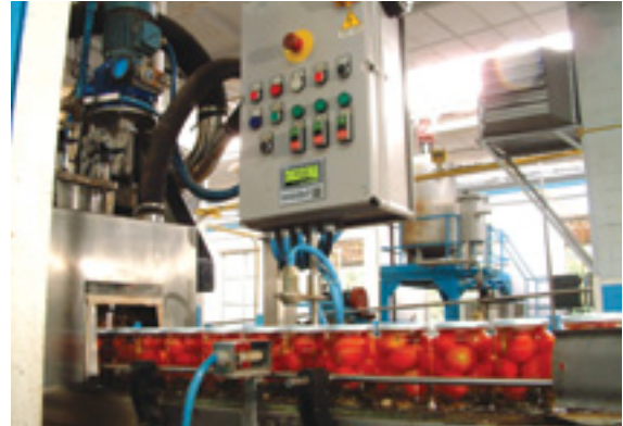
Moving parts on a filling machine can be hazardous without safe guards such as on/off push buttons.
